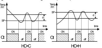
In the event of cell probe error (Pr1), it is possible to set the instrument so that that the output "Ot" continues to work in cycles according to the times programmed in the parameter (activation time) and "t2" (deactivation time).
