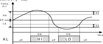
The maximum and minimum temperature alarms can be disabled by setting the relative parameters "HA" and "LA" = oF.
