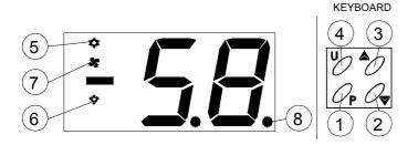
1 - Key P : Used for setting the Set point and for programming the function parameters
