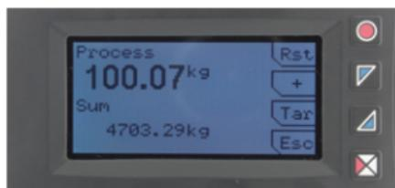
Press **[Sum Function]** to enter the function page. Pressing **[+]** the **Process** value is added to the counter. It is possible to reset the total value keeping pressed **[Rst]** and to fix "tare zero" of the process pressing **[Tar]**.
