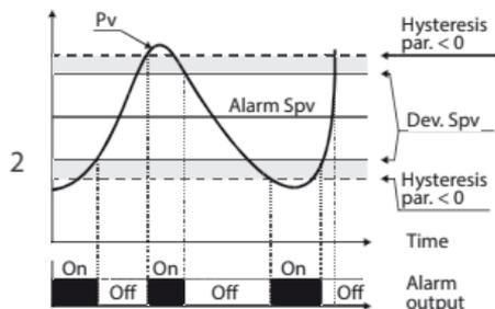
Band alarm and hysteresis value less than "0" (Par. 58 **hysteresis** < 0). N.B. The example refers to alarm 1; the function can also be enabled for alarms 2.
