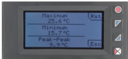
The STR550 is provided with a page for the visualization of peak values: max. peak, min. peak and peak-to-peak of analogue input. Keeping pressed **Rst** it is possible to reset the visualized values.
