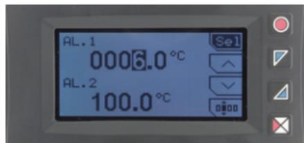
Press **Setpoint** to enter the thresholds modification.
