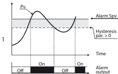
Absolute alarm and hysteresis value greater than "0" (Par. 58 **hysteresis** > 0). N.B. The example refers to alarm 1; the function can also be enabled for alarms 2
