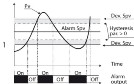
Band alarm and hysteresis value greater than "0" (Par. 58 **hysteresis** > 0). N.B. The example refers to alarm 1; the function can also be enabled for alarms 2.
