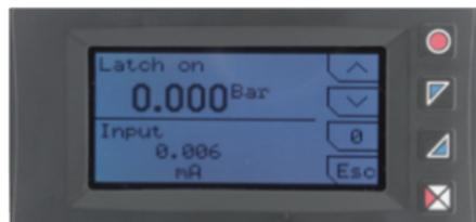
To use the LATCH ON function: enter configuration, select **Setting** on par. 8 **Latch on** and press **Sel** (STR550 shows the page in the picture).
