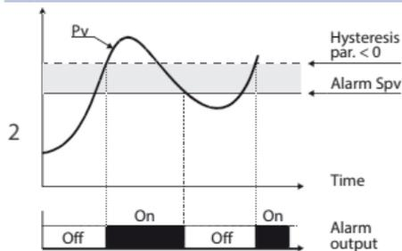
Absolute alarm and hysteresis value less than "0" (Par. 58 **hysteresis** < 0). N.B. The example refers to alarm 1; the function can also be enabled for alarms 2.
