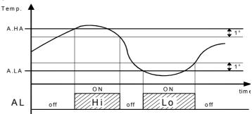
The alarm functions of the instrument work on the ALARM led, on or will be the values ["SP"+"A.HA"] and ["SP"+"A.LA"] if the alarms
