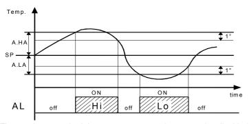
The maximum and minimum temperature alarms can be disabled by setting the relative parameters "A.HA" and "A.LA" = oF. The alarms histeresis (differential switching point) is fixed at 1°.
