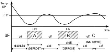
**Examples:** defrosting A ends due to reaching of temperature "dtE", defrosting B ends at the end of the "d.dE" time as the temperature "d.tE" is not reached, defrosting C does not take place as the temperature is higher than "d.tE".
