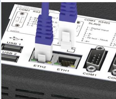
Two Ethernet 10/100/1000 Mbit ports on the rear side of the operator panel are available. ETH1 and ETH2 are internally connected to CPU through a Gigabit switch.
