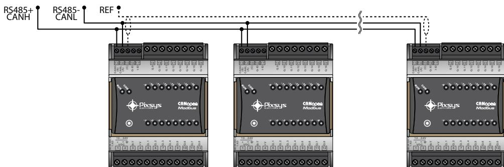
Below is the diagram for the connection of more than one MCM260X to a RS485 line or CAN network.
