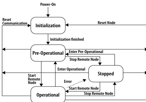
The NMT services allow the status to be changed in each condition. NMT messages are formatted by a CAN-header (COB-ID = 0) and 2 data byte. A byte contains the requested service (NMT command specifier) and the other contains the Node-ID (0 for broadcast mode). A CANopen network can only have an NMT master, which brings NMT messages and controls the initialization processes.
