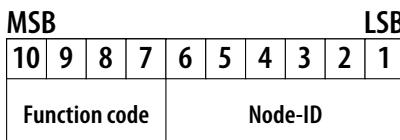
Pre-defined connection set defines 4 Rx PDO, 4 TX PDO, 1 SDO, 1 Emergency Object and 1 Node-Error-Control Identifier. It also supports the transmission in broadcast of NMT Module Control Services, SYNC and Time Stamp objects. The complete CAN identifier assignment scheme is shown below:
