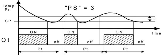
The function is disabled by programming "Pt" = 0. During the power on delay phases of the Ot output by inhibiting the function "Compressor Protection" the led OUT flashes. It is also possible to prevent activation of all the outputs after the instrument is turned on, for the time set in the parameter "od". The function is disabled by "od" = oF. During the power on delay phase, the display shows the indication od, alternating with the normal programmed visualisation.
