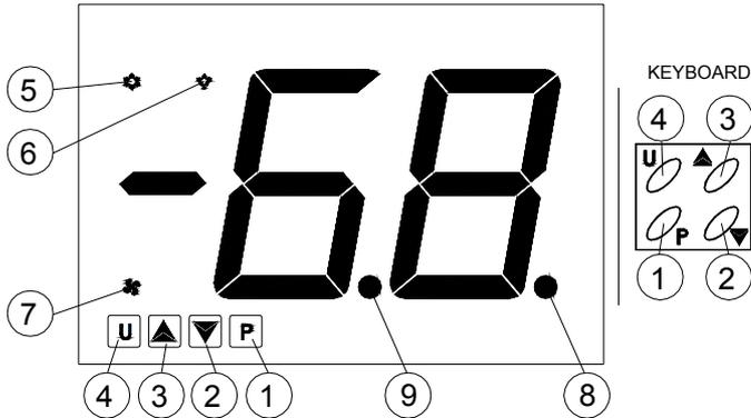
**1 - Key P** : Used for setting the Set point and for programming the function parameters
