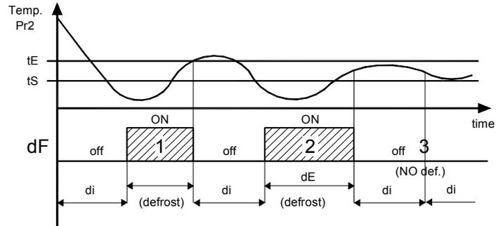
**Examples:** defrosting 1 ends due to reaching of temperature "tE", defrosting 2 ends at the end of the "dE" time as the temperature "tE" is not reached, defrosting 3 does not take place as the temperature is higher than "tS".
