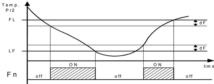
Notes: It is necessary to pay attention to the correct use of this fans temperature control functions because in the typical application of refrigeration the stop of the fans evaporator stops thermal exchange.
