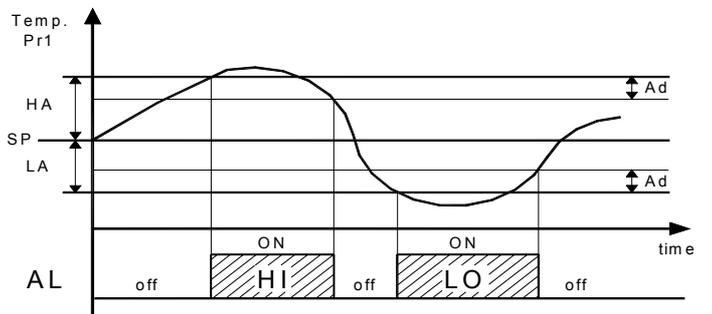
The maximum and minimum temperature alarms can be disabled by setting the relative parameters “HA” and “LA” = oF.
