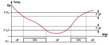
In fact it is possible disable the fans when the temperature measured by **EP** evaporator probe is higher than the one set at parameter F. FL (temperature too hot) or lower than the one set at parameter F.LF (temperature too cold).
