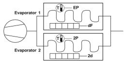
Schematic example of a two-evaporator system with electric defrost.
