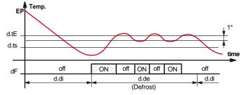
Example of electric defrost with evaporator temperature control: The defrost ends after d.dE programmed time. During defrost the **dF** output switch ON/OFF to control evaporator temperature in heating mode with set point d.tE and 1° differential (Hysteresis) in order to mantain the defrost temperature at the d.te set value.
