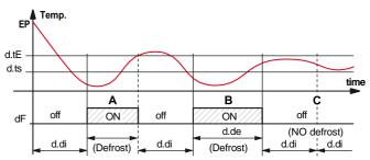
End defrost examples: defrost **A** ends due to reaching of temperature d.tE, defrosting **B** ends at the end of the d.dE time as the temperature d.tE is not reached, defrost **C** does not take place as the temperature is higher than d.tS.
