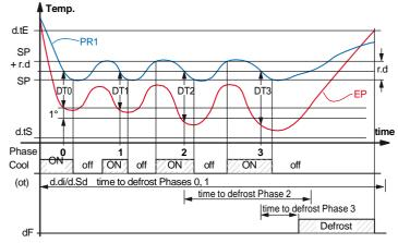
Example of *Dynamic defrost intervals system* with a reduction d.dd = 40% and end defrost by temperature.
