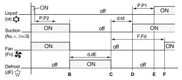
Example of **Hot Gas defrost for centralized systems** with defrost start when the *Liquid valve* is closed hafter the P.P2 time counting has expired.
