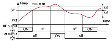
HC Cooling and Heating with two independent set points. Similarly, if parameter r.HC is programmed such that r.HC = HC, the output configured as **ot** operates with a cooling action (as r.HC = C) whereas the output configured as **HE** operates with a heating action (as r.HC = H). In this case the control Set Point for the **ot** output is the active one between **SP**, **SPE** and **SPH**, whereas the Set Point for the **HE** output is **SPH**.
