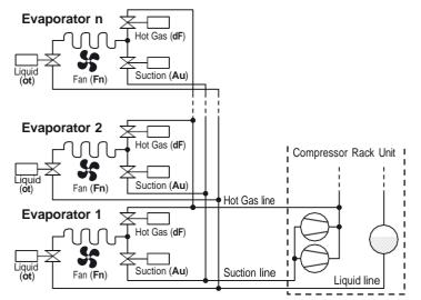
**Note:** For greater clarity in the diagram, some details concerning the hydraulic circuit have been deliberately omitted (non-return valves etc.) because they are not controlled by the instrument but are still necessary for the correct system operation.
