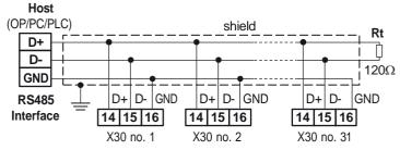
The interface circuit allows the connection of up to  ${\bf 32}$  instruments on the same line.
