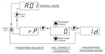
**Note:** If the Password gets lost, just swith off and on the instrument supply, push P key during the initial test and keeping the key pressed for 5 seconds.
