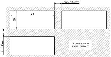
Y33 (instrument with mechanical keyboard) Y33S (instrument with Sensitive Touch keyboard)
