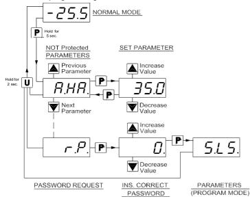
To make a parameter accessible without having to enter the password when "t.PP" password protection is activate follows this procedure.
