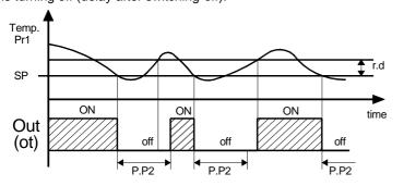
Third control (par. "P.P3") foresees an inhibition to the activation of the output "Out" by a time delay that starts when the output was turning on last time (delay between switching-on).
