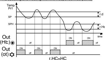
Similarly, if the parameter "r.HC" is programmed such that "r.HC" = HC, the output configured as "ot" operates with a cooling action (as "r.HC" = C) whereas the output configured as "HE" operates with a heating action.
