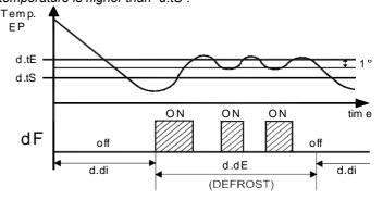
Example of electric defrost with evaporator temperature control: The defrost end after "d.dE" programmed time. During defrost the "dF" output switch on/off to control evaporator temperature in heating mode with set point "d.tE" and 1° differential (Hysteresis). The active defrost is shown on the instrument display with the lighting up of the DEFROST led
