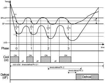
Example "dynamic defrost intervals system" with a reduction "d.dd" = 40 % and end defrost by temperature.
