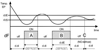
**Examples:** defrosting A ends due to reaching of temperature "dtE", defrosting B ends at the end of the "d.dE" time as the temperature "d.tE" is not reached, defrosting C does not take place as the temperature is higher than "d.tS".
