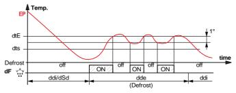
Example of electric defrost with evaporator temperature control: the defrost end after ddE programmed time. During defrost the **dF** output switch ON/OFF to control evaporator temperature in heating mode with set point dtE and 1° differential (Hysteresis).
