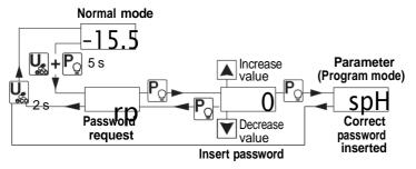
**Notes: 1.** All parameters are configured by default at "protected" level so that setting the tpp parameter protects all parameters with the password.
