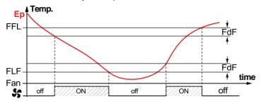
**Note:** Special attention must be paid to the correct use of the temperature-dependent fan control functions, as in a typical refrigeration application, stopping the evaporator fans blocks heat exchange.
