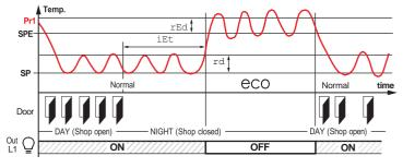
Example of automatic *ECO/Normal* mode activation. during the business hours the door is opened frequently and the controller remains in *Normal* mode. After the <code>iEt</code> time has elapsed since the door has not been opened anymore, the controller switches to *ECO* mode. As soon as the door is opened again, the controller returns to *Normal* mode.
