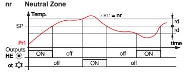
When rHC = nr, the output configured as **ot** operates with a cooling action (like rHC = C) while the output configured as **HE** operates with a heating action both with the Active Set Point (SP1, SP2, SP3, SPE or SPH). The intervention differential (rd/rEd/rHd) is automatically assumed by the controller to have positive values for the cooling action and negative values for the heating action.
