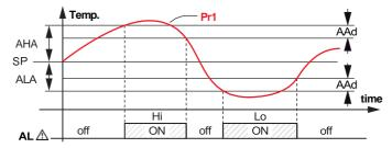
The maximum and minimum temperature alarms can be disabled by setting the related parameters AHA and  $\texttt{ALA} = \mathbf{oF}$ . The temperature alarms are signalled lighting up the alarm LED ( $\triangle$ ) and, if configured, also with the buzzer.
