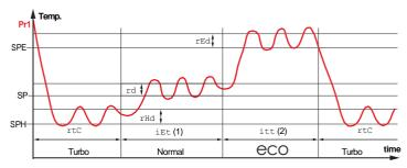
**Notes: 1.** The time iEt is reset every time the door is opened, in the case shown the door is always closed.
